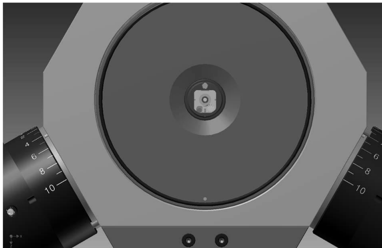
Figure 3-36 Specimen mount raised and in the Home position.
