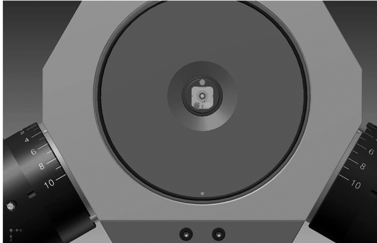
Figure 3-22 Properly aligned stage in the Home position
