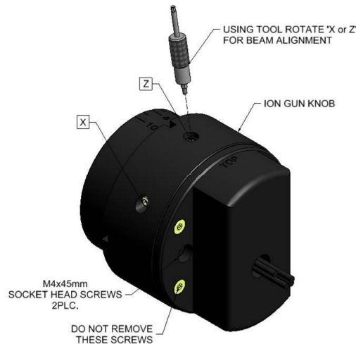
Figure 3-42 X and Z-alignment device screws
