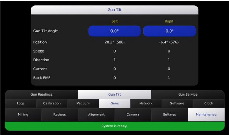
Figure 7-26 Gun tilt maintenance screen
