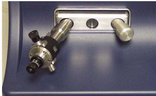
figure 11 TEM holder and adapter in place
