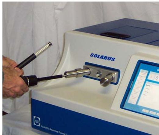
figure 10 Loading TEM holder, holder adapter, and plug
