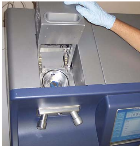
figure 13 Sample loaded in SEM chamber
