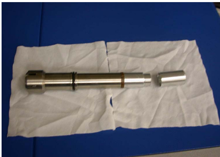
figure 14 TEM holder-adaptor with ion shield removed
