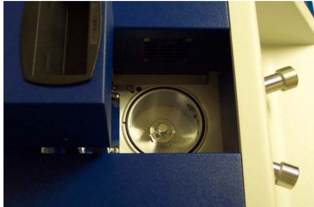
figure 12 Top-loading SEM chamber, side view
